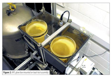
However, the use of a glove box precludes the transfer of artefacts directly from vacuum to vacuum. This is because the glove box transfer is carried out in an inert gas.
