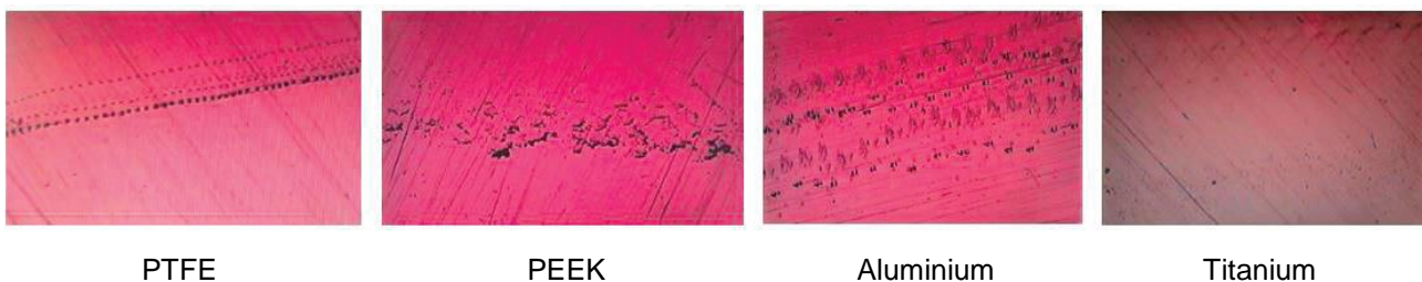
Figure 7: Effect of 5000 lifting cycles on a SS weight using pegs of the four materials indicated
