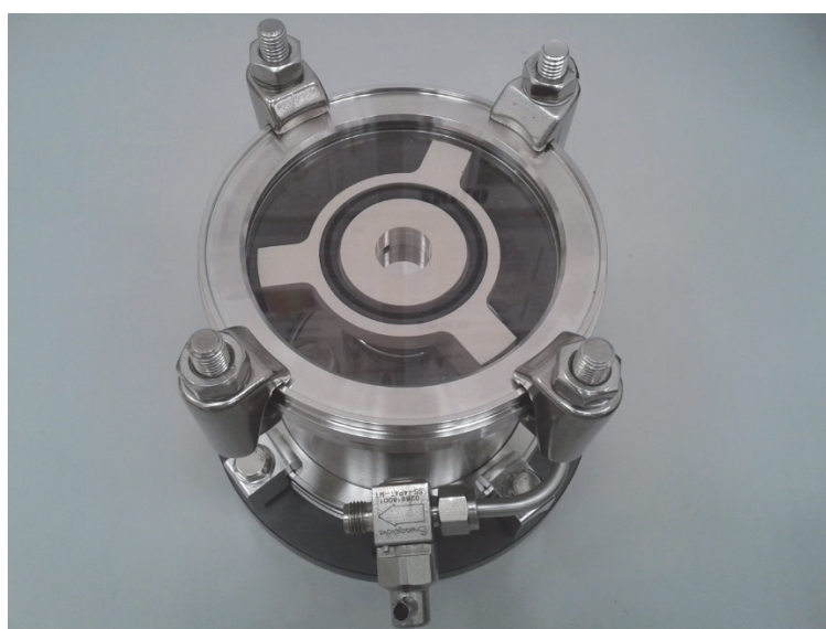
Figure 2. Stainless steel kilogram in an inert gas / vacuum compatible transfer vessel.
