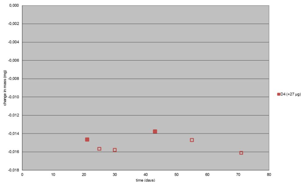
Figure 6: Change in mass of platinum-iridium standard during the BIPM nettoyage - lavage cleaning cycles. Data points with solid fill present the measurements after the cleaning cycle and data points with no fill present repeated measurements.
