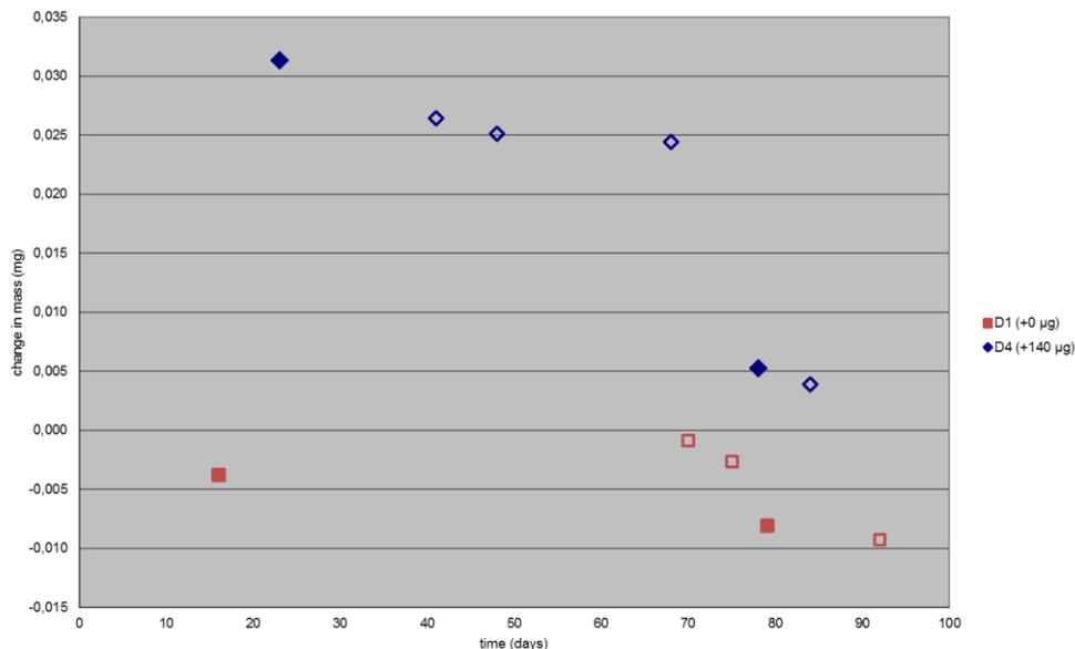
Figure 10: Change in mass of platinum-iridium standard during the UV/ozone cleaning cycles. Data points with solid fill present the measurements after the cleaning cycle and data points with no fill present repeated measurements.
