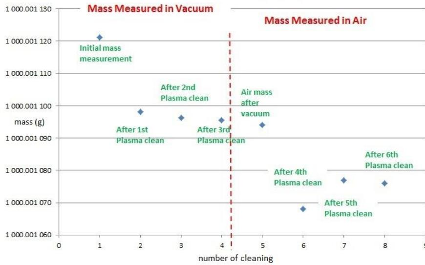
Figure 12: Change in mass of stainless steel standard LM006 during the hydrogen plasma cleaning cycles at NPL
