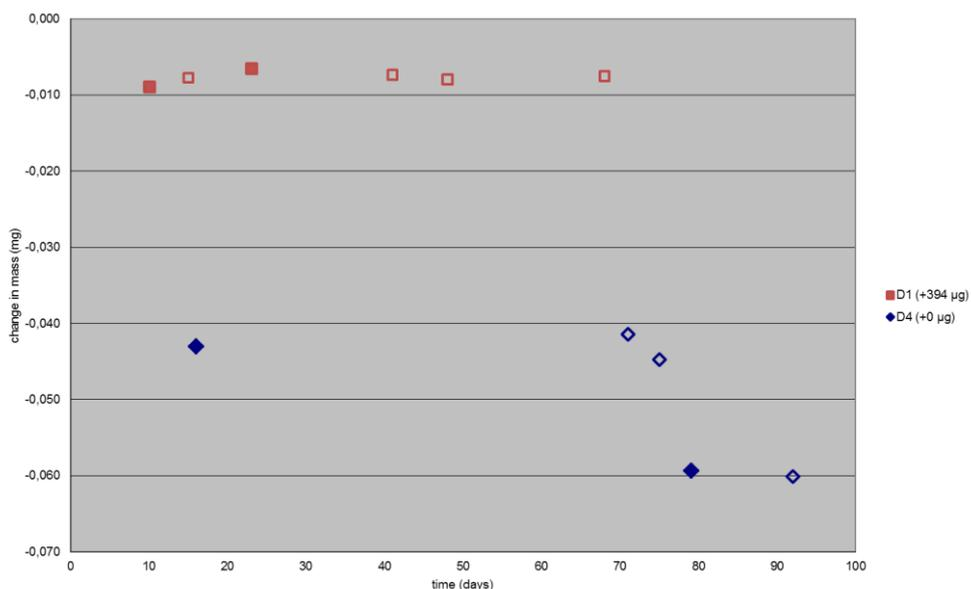
Figure 8: Change in mass of platinum-iridium standards during the ultrasonic bath cleaning cycles. Data points with solid fill present the measurements after the cleaning cycle and data points with no fill present repeated measurements.
