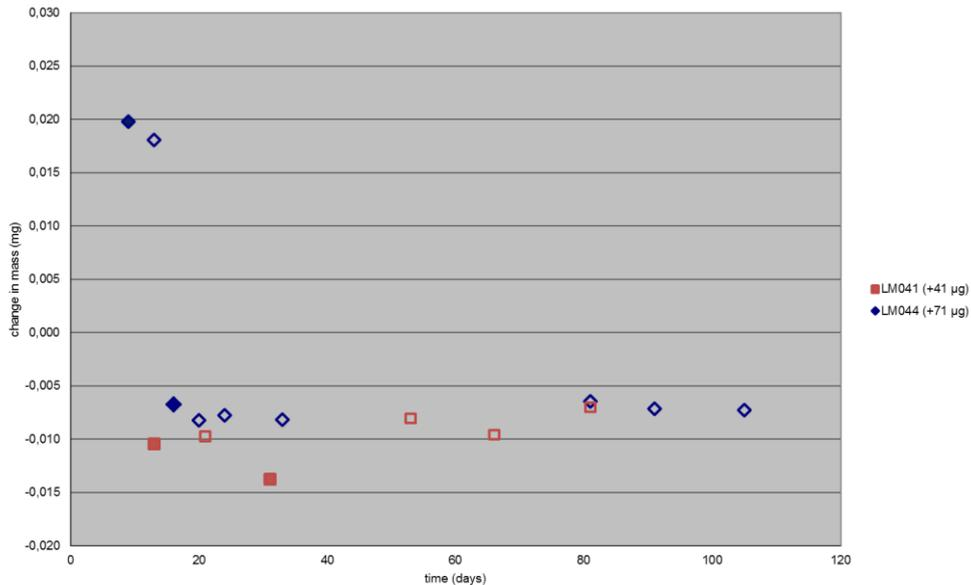
Figure 7: Change in mass of stainless steel standard during the ultrasonic bath cleaning cycles. Data points with solid fill present the measurements after the cleaning cycle and data points with no fill present repeated measurements.
