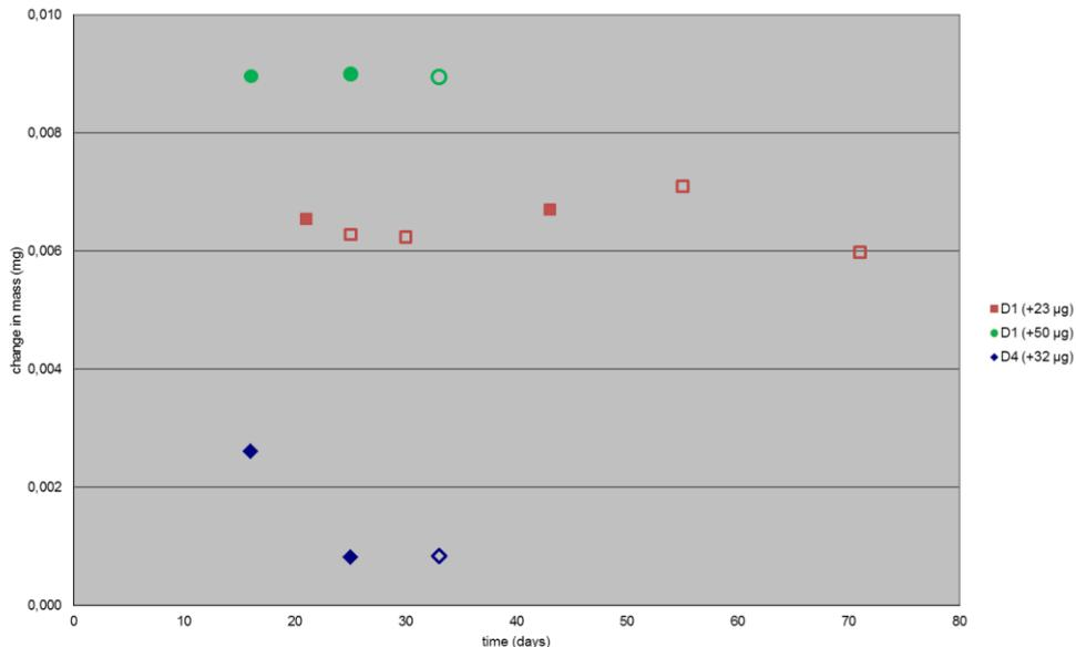
Figure 13: Change in mass of platinum-iridium standards during the hydrogen plasma cleaning cycles. Data points with solid fill present the measurements after the cleaning cycle and data points with no fill present repeated measurements.
