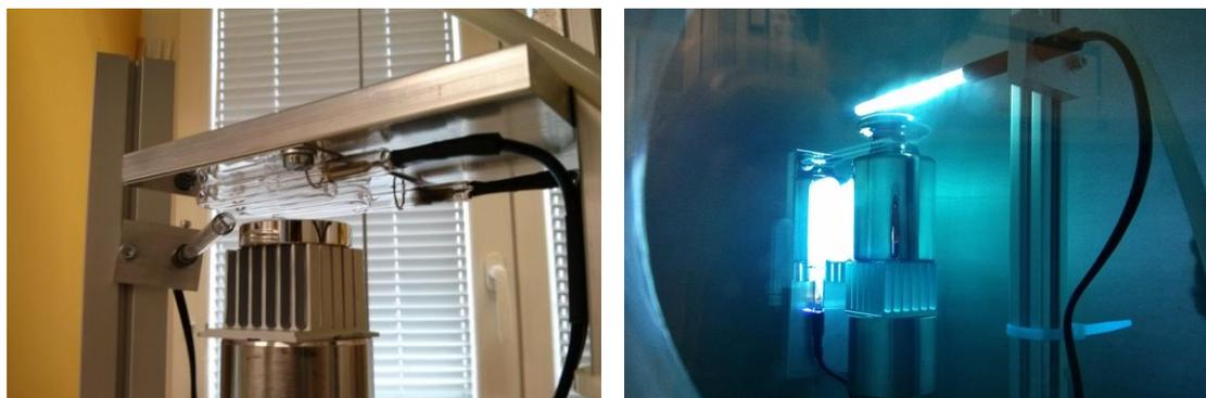
Figure 3: Platinum - iridium disc standard (left) and stainless steel standard (right) in the UV/ozone apparatus
