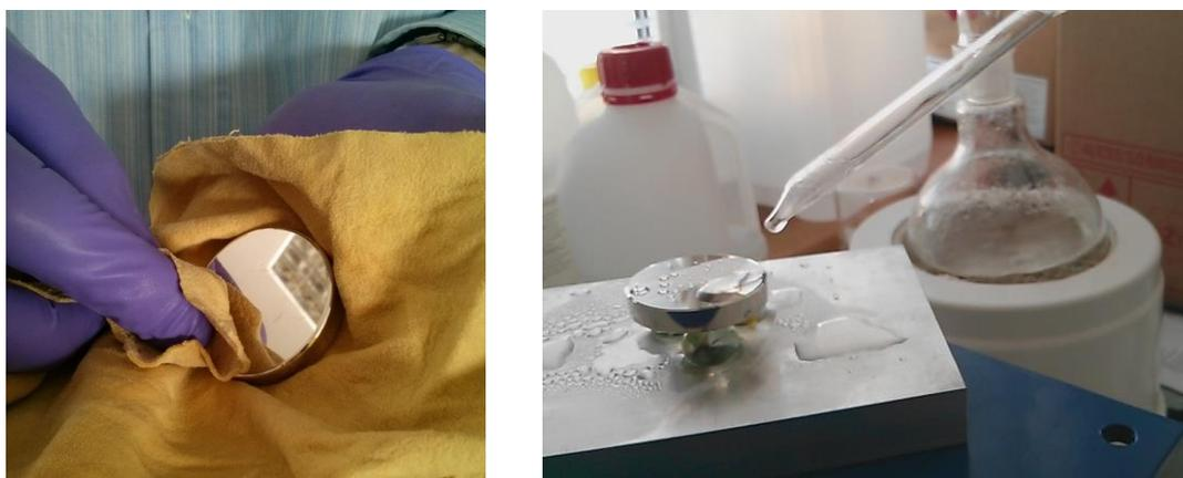
Figure 1: Cleaning with chamois leather cloth soaked in ether-ethanol mixture (left) and washing with bidistilled water steam jet (right).
