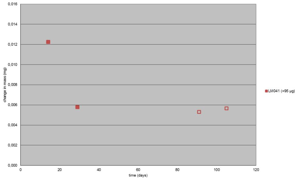
Figure 5: Change in mass of stainless steel standard during the BIPM nettoyage - lavage cleaning cycles. Data points with solid fill present the measurements after the cleaning cycle and data points with no fill present repeated measurements.
