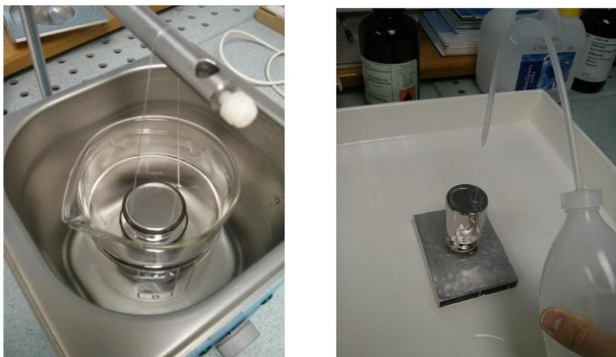
Figure 2: Cleaning in the ultrasonic bath (left) and rinsing with bidistilled water (right).
