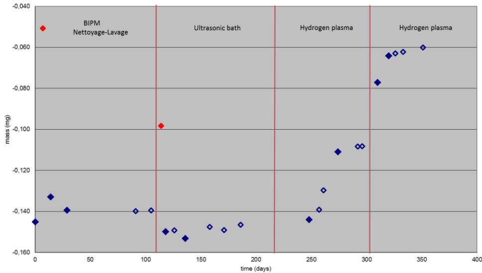
Figure 15: Deviation from nominal mass of stainless steel standard (LM-041) during the sequence of different cleaning procedures. Red data points present measurements after applied contamination (data point for plasma cleaning cycles are off the chart, - 0,017 mg, + 0,019 mg), blue data points with solid fill present the measurements after the cleaning cycle and blue data points with no fill present repeated measurements.
