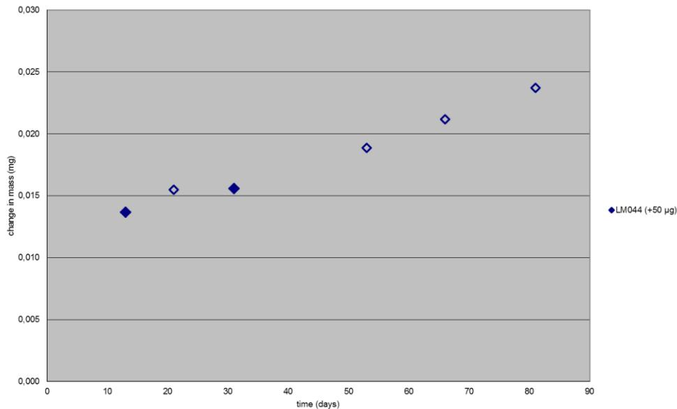
Figure 9: Change in mass of stainless steel standard during the UV/ozone cleaning cycles. Data points with solid fill present the measurements after the cleaning cycle and data points with no fill present repeated measurements.
