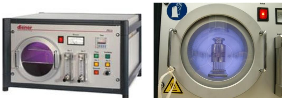
Figure 4: Diener Pico plasma system (left) and cleaning of stainless steel standard with hydrogen plasma (right).
