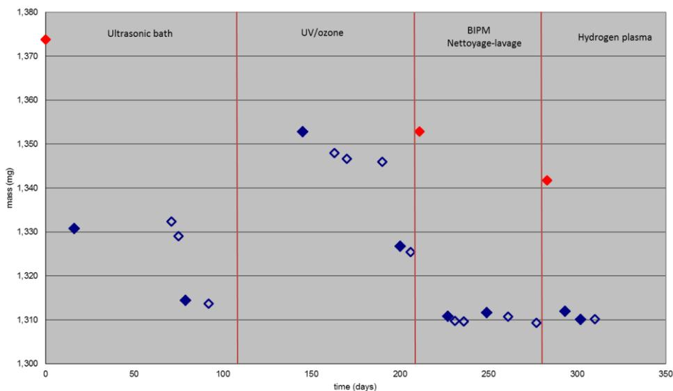
Figure 14: Deviation from nominal mass of platinum-iridium standard (D4) during the sequence of different cleaning procedures. Red data points present measurements after applied contamination (data point for UV/ozone is off the chart, + 1,466 mg), blue data points with solid fill present the measurements after the cleaning cycle and blue data points with no fill present repeated measurements.
