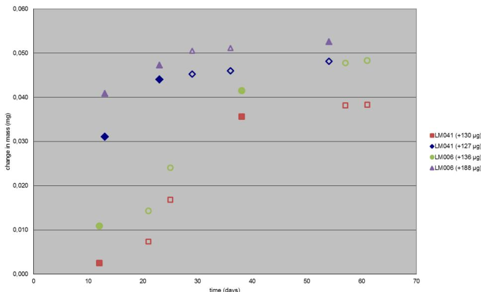
Figure 11: Change in mass of stainless steel standards during the hydrogen plasma cleaning cycles. Data points with solid fill present the measurements after the cleaning cycle and data points with no fill present repeated measurements.
