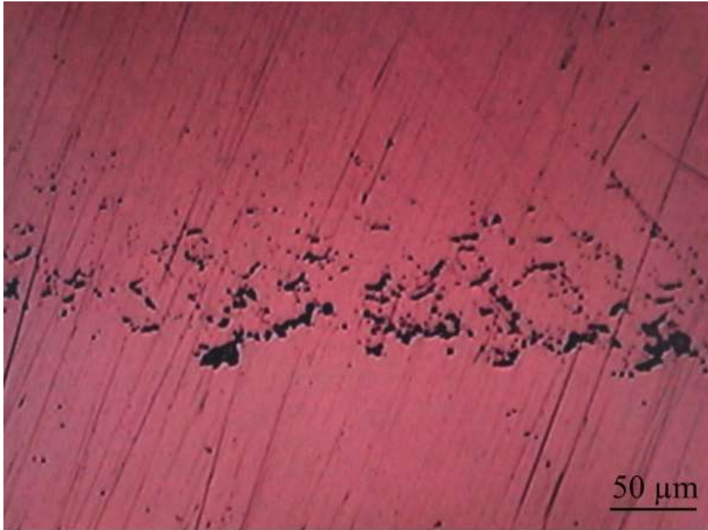
Figure 20. Optical microscope image of the contact area for PTFE.
