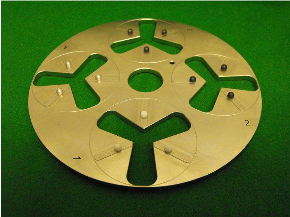
Figure 1 Modified turntable of the HK1000 mass comparator fitted with the test pegs manufactured from the support materials.
