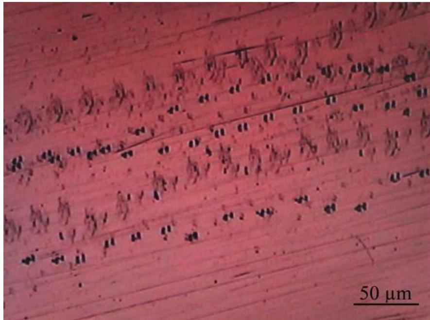
Figure 18. Optical microscope image of the contact area for aluminium.
