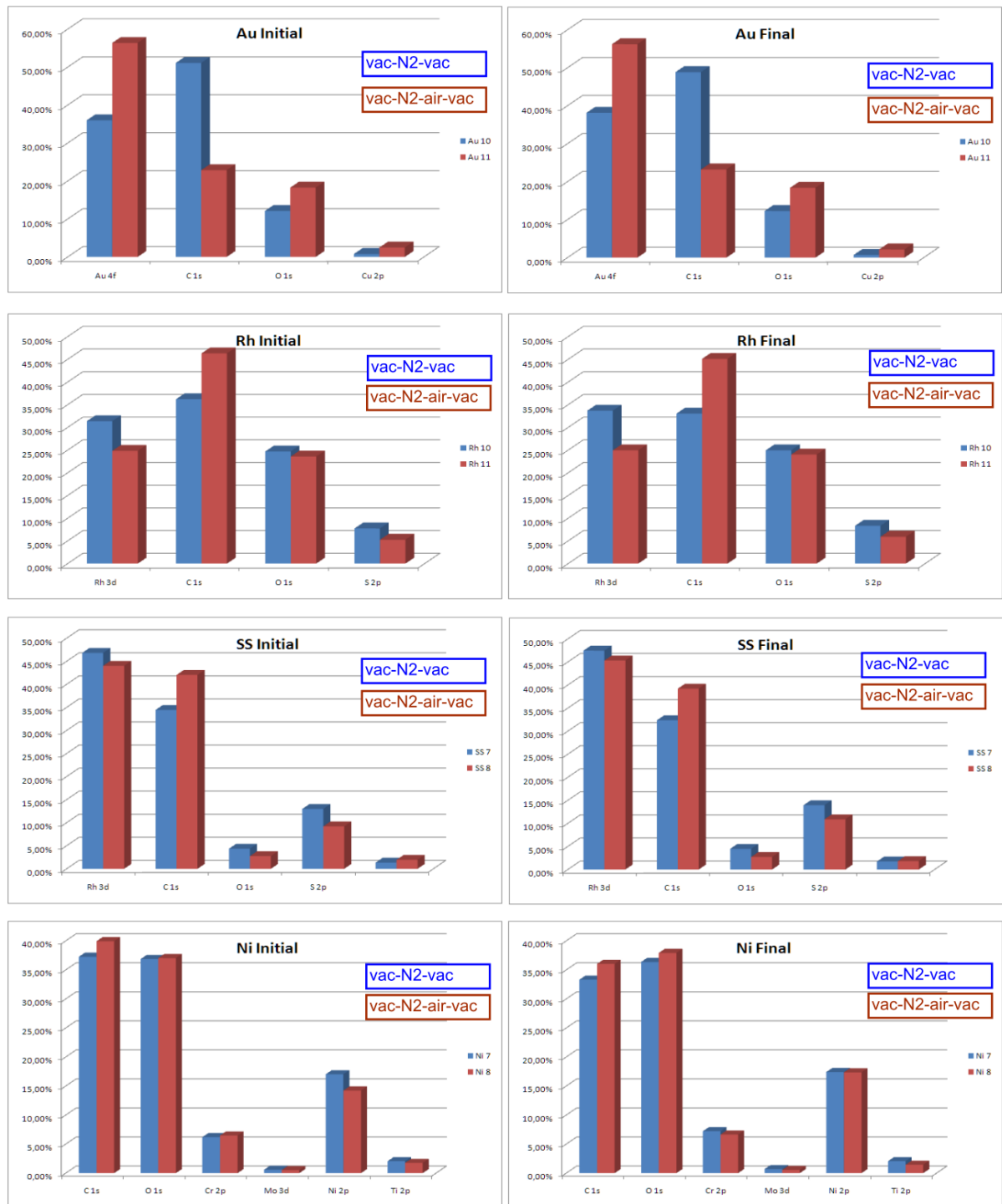
Figure 11: Percentile comparison of initial (left) and final (right) surface composition on stainless steel, Ni-alloy, electroplated Au and electroplated Rh for the venting processes vacuum-N 2 -vacuum and vacuum-N 2 -air-vacuum (data from TUBITAK).
