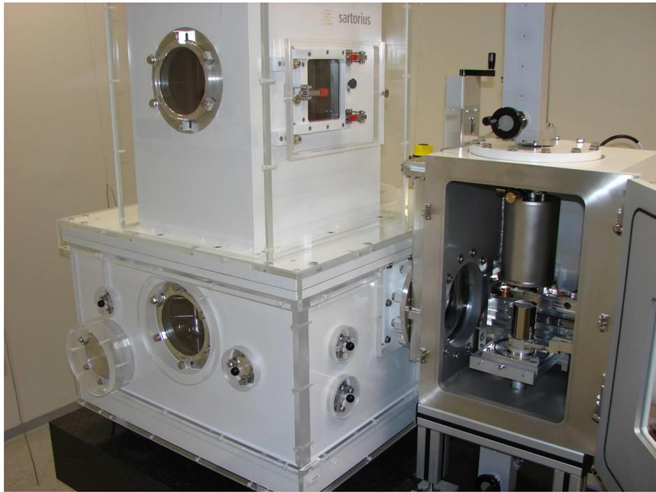
Figure 3 : PTB CCL1007 vacuum comparator
